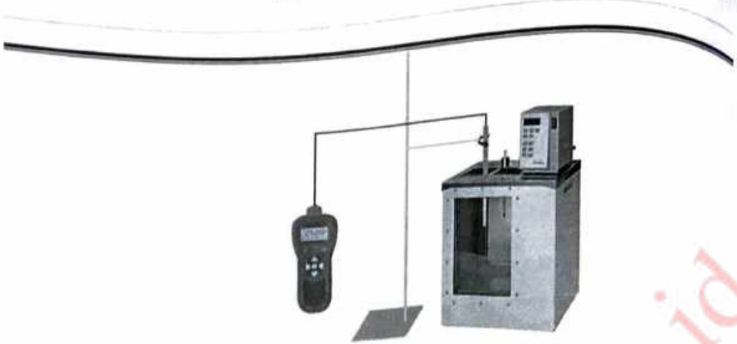
Gambar 4 Set-up Kalibrasi thermometer klinik
